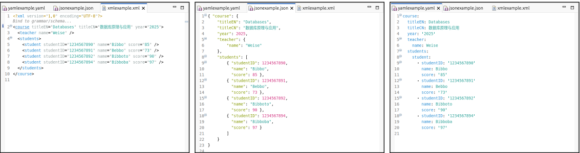
(1.3.1) An example of data stored in the Extensible Markup Language (XML). (1.3.2) An example of data stored in the JavaScript Object Notation (JSON). (1.3.3) An example of data stored in the YAML Ain't Markup Language™ (YAML).
